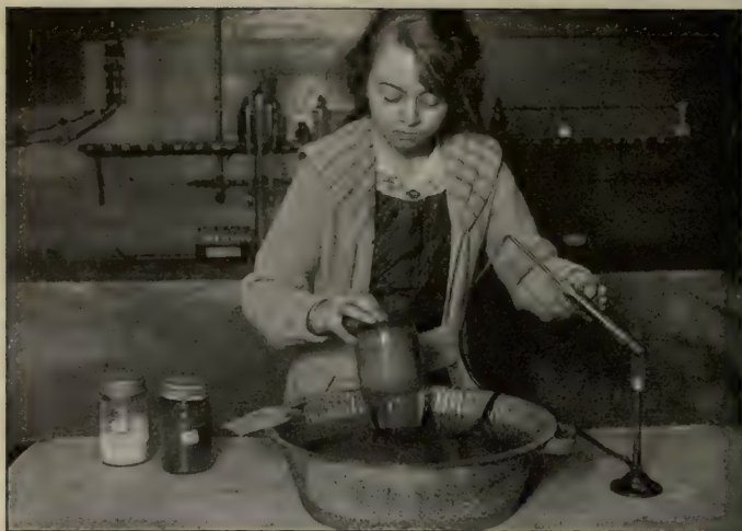
FIG. 165. Filling a bottle with oxygen.
